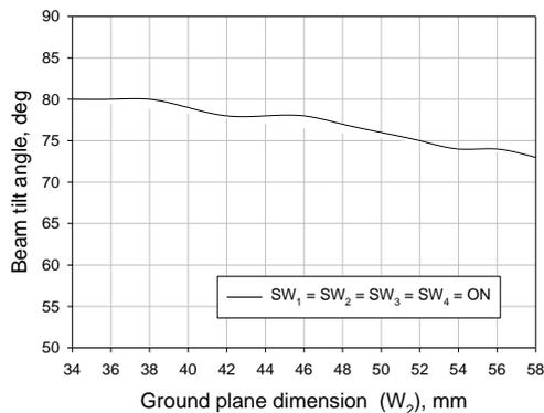
Fig.10. Variation of ground plane ( $W_2$ ) with beam tilt angle
