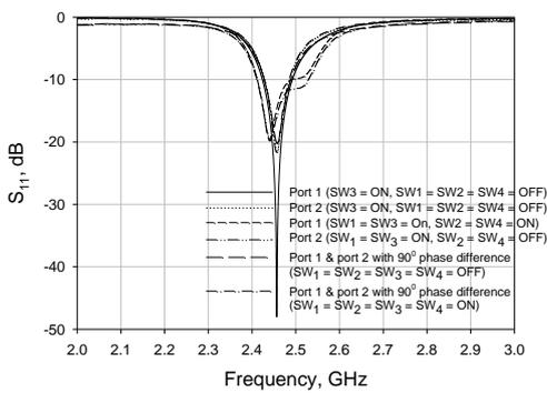
Fig.2. Simulated reflection coefficient of the antenna for different switching conditions
