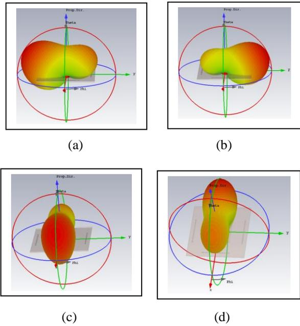
Fig.6. 3D radiation pattern (a)  $SW_3 = ON, SW_1 = SW_2 = SW_4 = OFF$  (b)  $SW_1 = ON, SW_2 = SW_3 = SW_4 = OFF$  (c)  $SW_2 = ON, SW_1 = SW_3 = SW_4 = OFF$  (d)  $SW_4 = ON, SW_1 = SW_2 = SW_3 = OFF$
