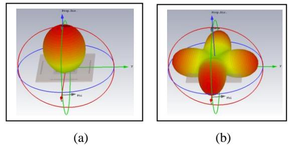
Fig.4. 3D radiation pattern (a)  $SW_1 = SW_2 = SW_3 = SW_4 = OFF$  (b)  $SW_1 = SW_2 = SW_3 = SW_4 = ON$
