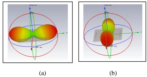
Fig.5. 3D radiation pattern (a)  $SW_1 = SW_3 = ON$ ,  $SW_2 = SW_4 = OFF$  (b)  $SW_1 = SW_3 = OFF$ ,  $SW_2 = SW_4 = ON$
