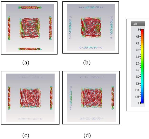
Fig.7. Surface current distribution (a)  $SW_1 = SW_2 = SW_3 = SW_4 = ON$  (b)  $SW_1 = SW_2 = SW_3 = SW_4 = OFF$  (c)  $SW_1 = SW_3 = SW_4 = ON, SW_2 = SW_4 = OFF$  (d)  $SW_3 = ON, SW_1 = SW_2 = SW_4 = OFF$
