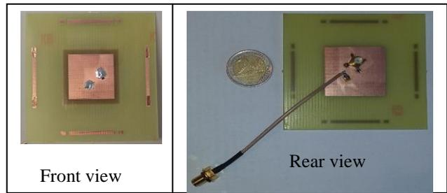
Fig.8. Photograph of the fabricated antenna
