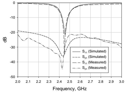
Fig.3. Simulated and measured reflection coefficient  $|S_{11}|$  and port isolation  $|S_{21}|$
