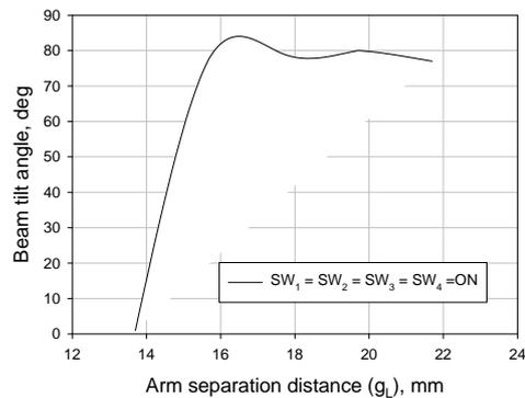
Fig. 9. Variation of arm separation distance ( $g_L$ ) with beam tilt angle
